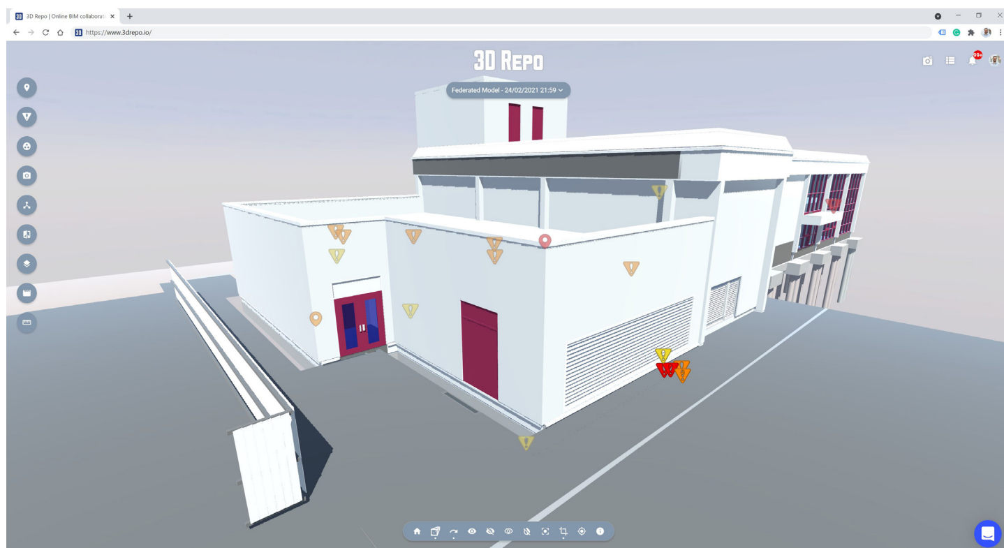
Figure 3: A different angle showing the AstraZeneca Macclesfield model in the 3D Repo platform. Coloured pins represent potential issues and risks.
