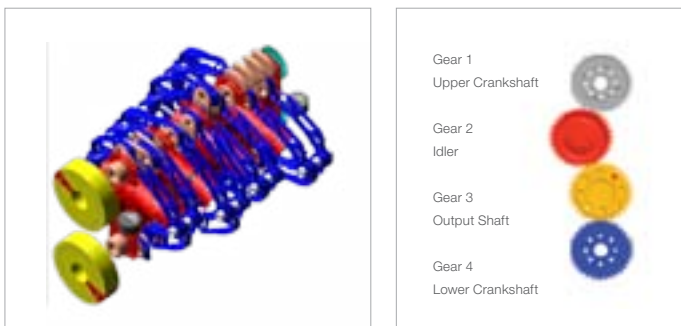
Figure 1: FEV Virtual Engine (powered by Adams) Crank Train model with Flexible Components and Rear View of the Gear Train
