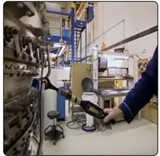
The IQWrench2 digital torque wrench in use during jet engine production audits, testing the torque applied to critical fasteners.
