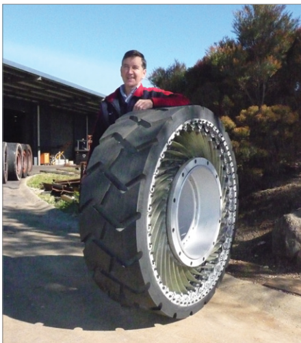
Fig. 1: Inventor Bruce Loudon with non-pneumatic non-solid wheel prototype
