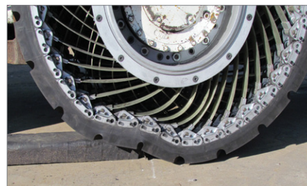
Fig. 7: Picture of prototype wheel advancing over an obstacle
