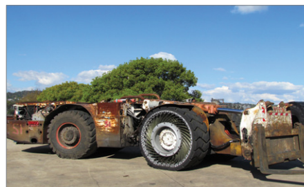
Fig. 2: Picture of Underground Mining Machine (Eimco 913) with Big Tyre's first full-size prototype wheel
