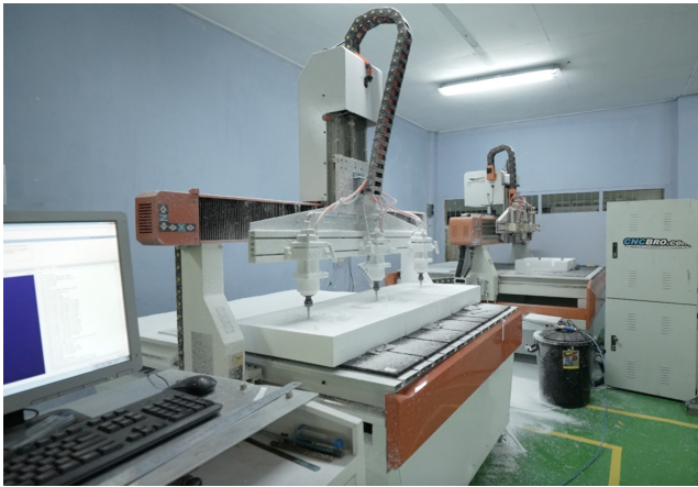
In-house EPS Foam Processing and Production
