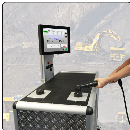
An example of our innovative tJRS joint simulator benches, available in ranges from up to 1000Nm.
