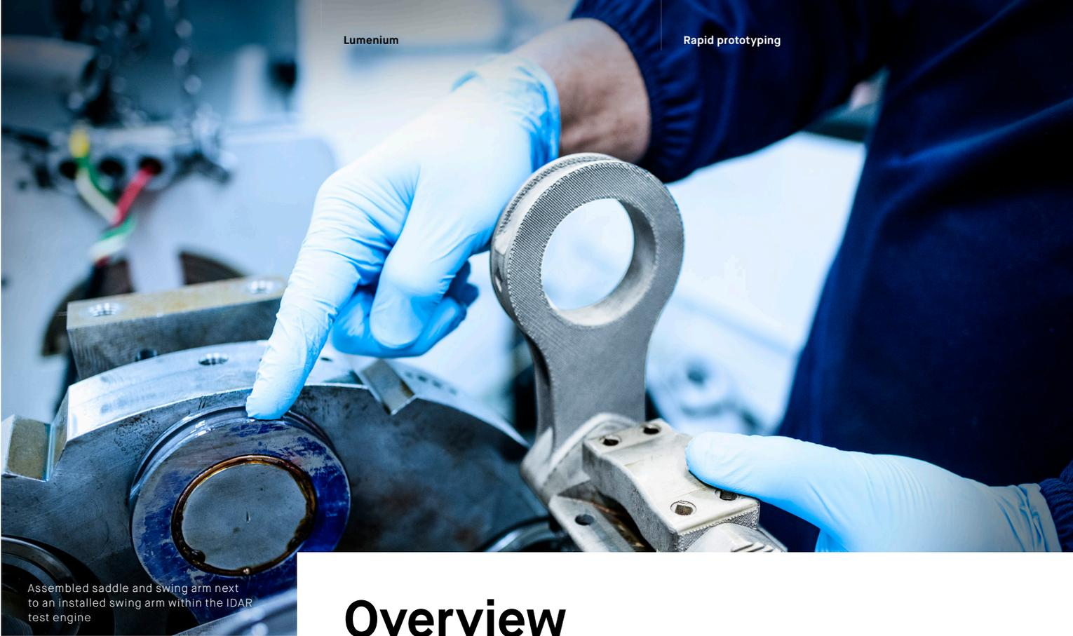
Assembled saddle and swing arm next to an installed swing arm within the IDAR test engine
