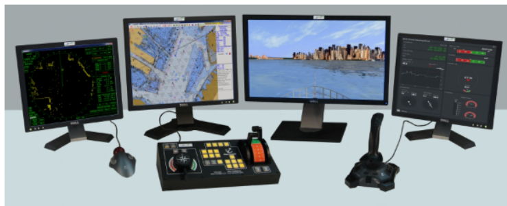
Desktop Ship Simulator with Tabletop Console
