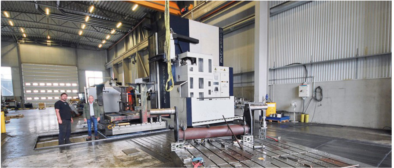
The Soraluce FR-12000 milling machine has twin rotating 60-tonne feed beds, offering six-axis machining.
