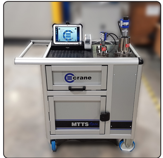
The bespoke MTTS trolley supplied to LEVC including the toughpad with built-in OMS software, label printer, Static and Rotary transducers, driven by the built-in TorqueStar data collector, hidden within the trolley.
