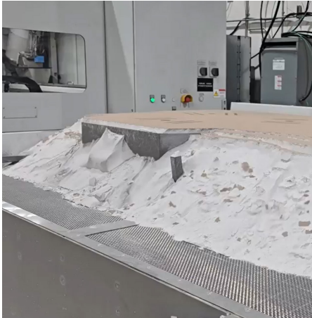
Mold packages are 3D printed in sand from a digital file, removed from the job box, assembled and prepped for casting without traditional tooling or core boxes.
