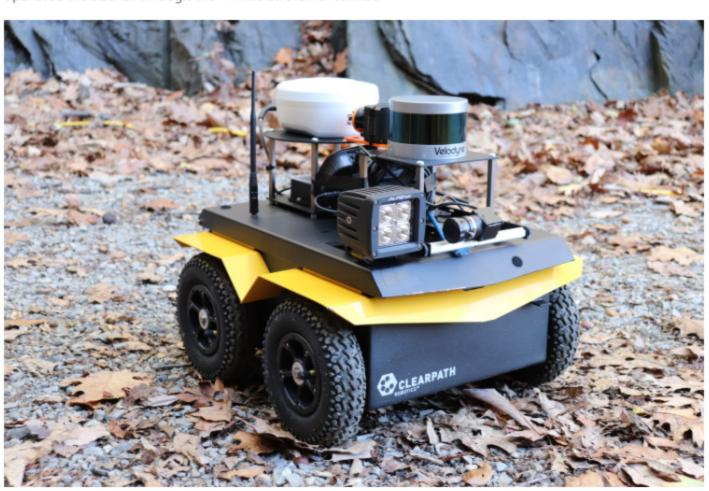
"Jackal UGV provided ample payload capacity, computing power and battery life without sacrificing portability. Its compact size allowed us to easily transport the robot to and from the tunnel, with very little setup required onsite." says Bezzo. "On top of that, its rugged build and waterproof chassis allowed us to operate in rocky and wet areas within the tunnel without disruption."
