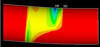
Plot shows non-uniform contact pressure distribution between shaft and bushing, enabling engineers to accurately calculate bushing wear rates and thus guide decisions on selection of component materials and surface finishes to maintain overall reliability of the fitness equipment.
