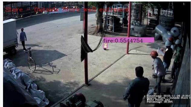
***Industrial AI platform detects a fire and identifies its location, triggering real-time alarms and alert notifications.***
