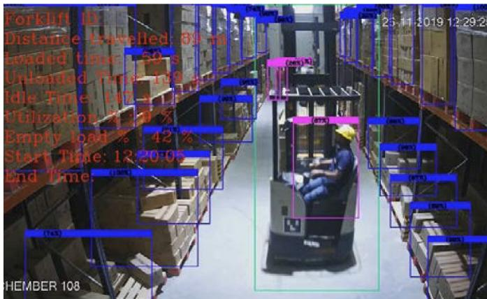
*Avathon Industrial AI platform can track and analyze forklift usage as well as the safety and efficiency of storage/stacking practices.*
