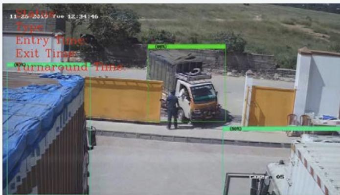
**Cameras running Industrial AI platform track each vehicle on-premises, monitoring factors related to turnaround time and labor time required for loading and unloading.**
