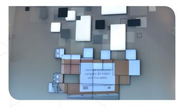
AVI enhanced collaboration in the Solution Lab by creating a 14-foot-long video wall made up of 7 MultiTaction displays – the only technology capable of providing full interactive capability on a curved wall. Whether the presentation involves videos, PDFs, web pages or video conferences, the presenter can easily pull up elements through video switching and distribution software.
