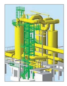
Large vessels, tanks, reactors and a high number of pipelines are characteristic for chemical plants. In general the pipes are essential components of large-scale technical plants, even in refineries or power stations, since they are required for interconnection of components, for supply and discharge of fluids.
