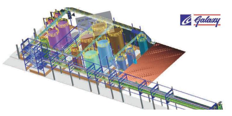
The project was executed by 3 engineers who were allocated defined areas of work. The engineers completed the equipment modeling, steel layout, pipe routing, etc. in a separate database and later merged them into a single database.
