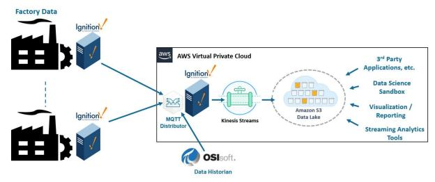
With so many edge sites and data sources in the deployment, the MQTT modules from Cirrus Link are essential to take Ignition tags and convert them to MQTT / Sparkplug, send them upstream, and then convert them back to Ignition tags for the central system in the cloud. This scalable solution converts OT data from all facilities to IT data, pushes it to the central system in a standard interface for data consumers, and then into data lakes for further analytics.
