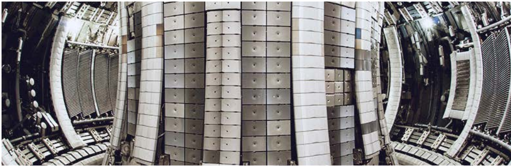
The tokamak is an experimental machine designed to harness the energy of fusion. ITER will be the world's largest tokamak. The image shows the inside of the JET machine at CCFE, UK.
