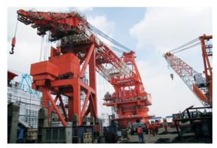
An innovative 3000-tonne derrick pipe-laying barge built by Shanghai Zhenhua Heavy Industry Co., Ltd.\* uses the world's most advanced pipe-laying technology. The vessel's 3000-tonne, 360° slew crane is driven by VACON® AC drives.
