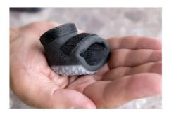
Once satisfied with the design, it was 3D printed on 3D Systems' multi-material **Projet MJP 5600** 3D printer. This printer enables both flexible and rigid materials to be printed and blended simultaneously at the voxel level for custom strength and elasticity. The resulting boot achieved the intended effect in durability, weight and fit, enabling Purps to walk and swim like the rest of her peers.
