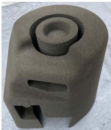
Production 3D printing applications delivered from Hoosier Pattern ready for casting at Decco.
