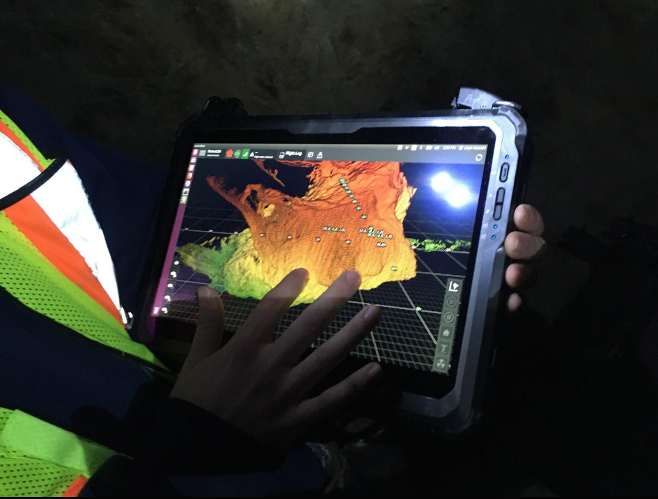
Manipulating 3D data collected from the stope in real-time, during the flight.
