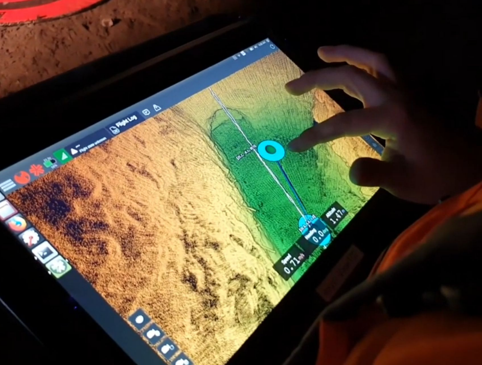
Manipulating 3D data collected from the slope in real-time, during the flight.
