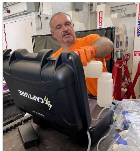
Fig. 1 - TRS operator running a field test using the FRED-PFAS kit.
