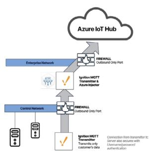
The Ignition Edge Server - acts as the MQTT transmitter at the contract manufacturing plant, gathering on Janssen's key process data directly from the control system and publishing it on the change through an outbound-only port on the control network firewall to the MQTT server. The connection is also secured via user authentication.
