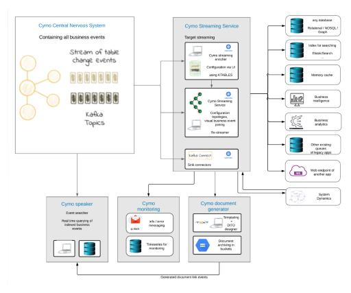
The redesigned Cymo architecture, showing how the different components are connected using its streaming architecture.
