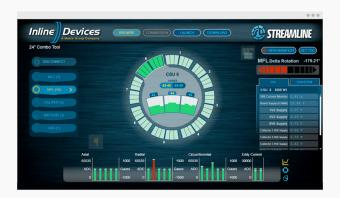
Atomic provided embedded software development for Microline's Atomic provided embedded software development for Microline's 24-inch Smart PIG, and Windows app development for Streamline, created using C# in WPF. Atomic also developed an open source tool for communication among different parts of the system and a simulation framework so the team could test Streamline with real
