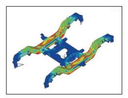
The analysis procedures used by Bombardier have been developed over a number of years, and output from one analysis tool is regularly used as input for another. MSC.Nastran results are postprocessed with MSC.Patran and Bombardier uses the static results as input to their own fatigue tools. Bombardier plans to harmonize fatigue tools in a next phase. One of the impediments to fatigue harmonization is the fact that so many different international and national standards are involved.
