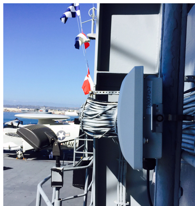
ABOVE: Ruckus ZoneFlex T301s provide sectorized antenna systems to extend and strengthen signals across the 4-acre outdoor decks on the USS Midway.
