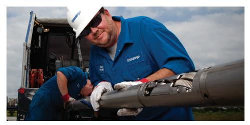
The bidirectional TuffTRAC tractor provides large pull and push forces that are precisely controlled from the surface. Sensors incorporated in the tractor enable the engineer to monitor tractor response and the progress of downhole operations while controlling the tractor for optimal performance.
