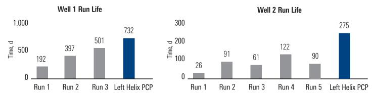
Average run life in Well 1 more than doubled after Schlumberger installed a Left Helix PCP to reduce plugging from sand production. The Left Helix pump restored production and more than tripled the average PCP run life in Well 2, which had been shut in for nearly 1 year because of the economics of repeatedly replacing conventional PCPs plugged by the more extreme sand production.
