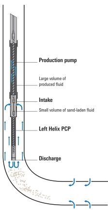
The Left Helix pump design incorporates a bottom rotor to pump a small percentage of fluid downward, which prevents sand accumulation at the intake. The design also replaces the conventional bottom tag with a top tag to reduce plugging risks.
