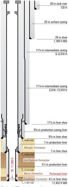
The Neyrfor TTT turbomill successfully removed scale buildup from the 4½-in production liner, enabling Ecopetrol to access the Mirador and Barco formations.
