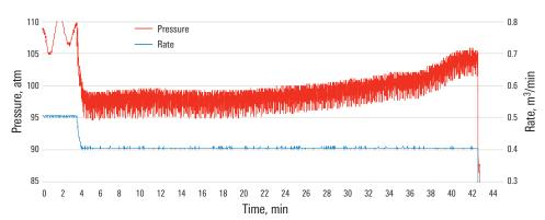
When the diversion pills entered a natural fracture or loss zone, the pressure increased. This indicated the impermeable particles diverted the treatment away from the fracture and into lower-permeability areas.
