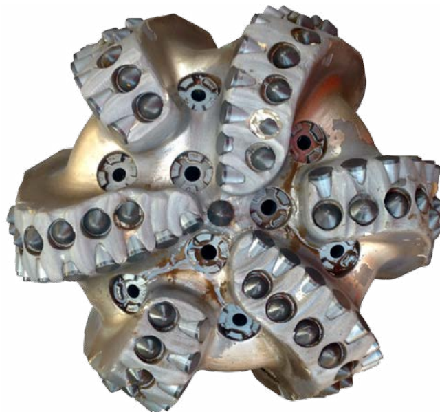
The cutters on both the bit and the reamer showed little to no wear.
