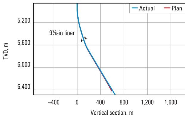
*The PowerDrive ICE RSS built the inclination of the well from 17.5° to 26.3° and maintained the tangent in automatic hold mode, making it possible to reach both intended targets in the HT reservoir.*
