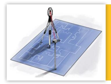
The Triple 'M' crews download the hanger locations to the Trimble MEP Layout Solution for use in the field. The robotic solution allowed the team to locate all hanging bracket locations in one day and then drill and install the hangers the following day.
