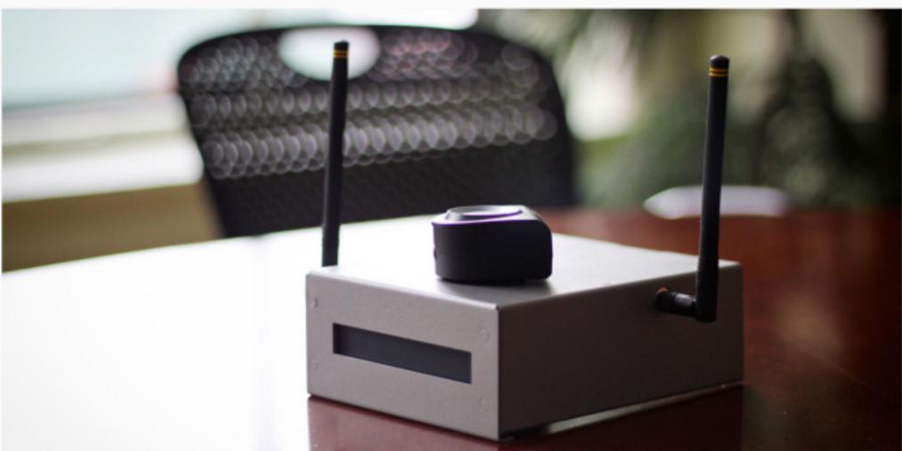
The patented wireless data collection system gathers data from hundreds of sensors via wireless networks, then compresses it and sends it to a central database, where it can be analyzed via an interactive web app.
